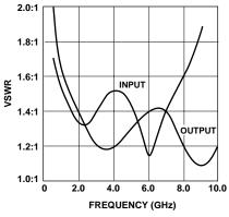
Figure 4. VSWR vs. Frequency, V<sub>d</sub> = 10 V.
